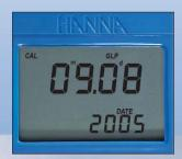
The HI 96 series of photometers displays the last time calibration was performed so you may schedule routine calibrations—ideal for ISO and Good Laboratory Practice environments.
